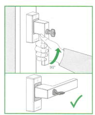
In the closed position (0° position) the window handle can be locked with a key and thus has an additional burglar-resistant security function. Only by unlocking (turning the key) can the handle be brought into the tilt position (90° position).
